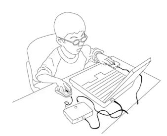
**Fig. 2** A child with cerebral palsy operates a mouse via an Integrated Pointing Device Apparatus. The child uses the mouse for cursor control with his dominant hand and uses an external switch for click control with the other hand simultaneously.
