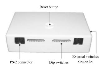
Fig. 1 Integrated pointing device apparatus hardware.
