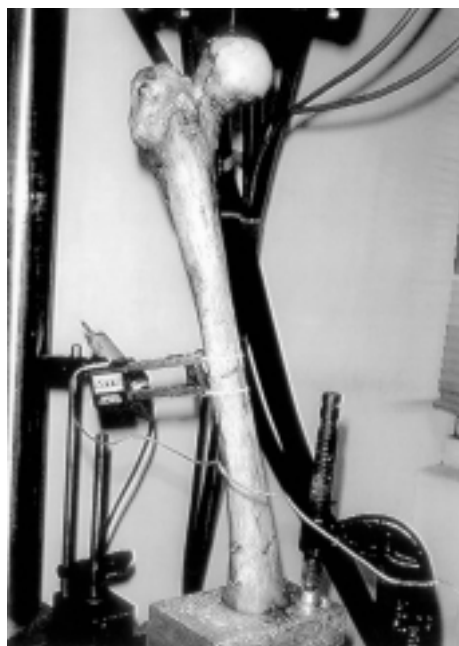
Fig. 2 The entire femur was mounted in a uniaxial Bionix 858 Material Testing System (MTS) machine for mechanical testing. An extensometer was placed at the lateral aspect of fracture fragments to measure the relative displacement of fragments.
