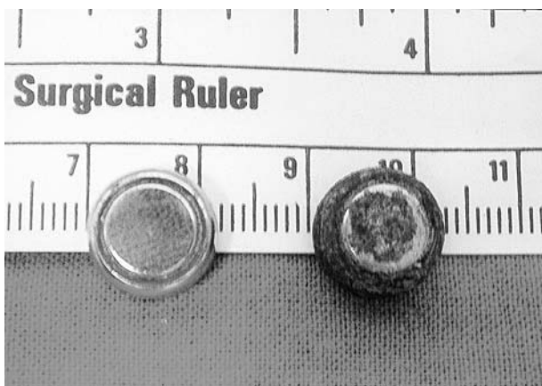
Fig. 2 A battery removed by endoscope (right) with corrosive dissolution in a child with gastric disc battery ingestion, compared with a normal battery (left).
