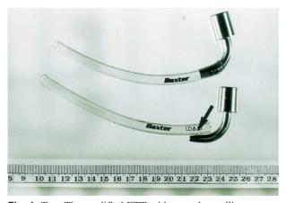
**Fig. 1** Top: The modified ETT with a steel metallic connector. Bottom: The damaged tube with bite imprints (arrow), deformed and flattened opening of the metallic connector.
